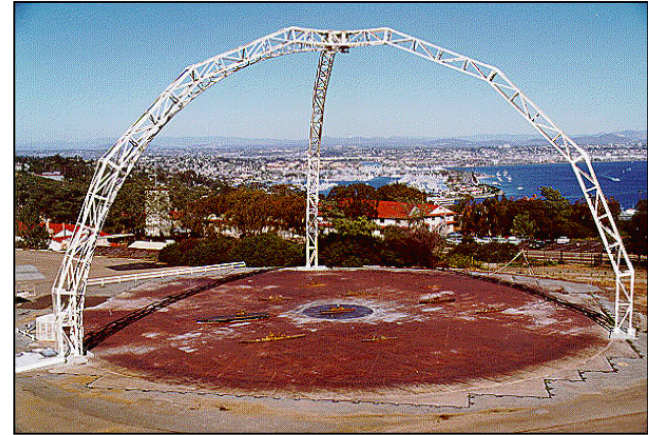
Scale Model Pattern Range 360° Azimuth, 3° - 90° elevation cuts 1 - 30 MHz amplitude and phase
