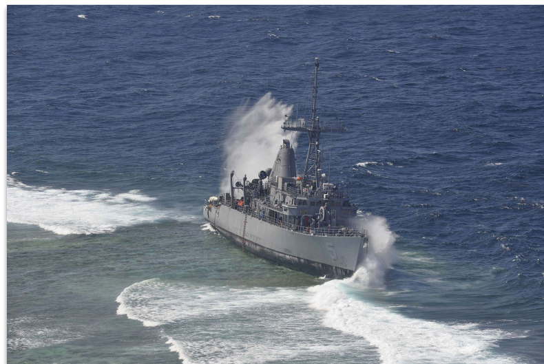
USS Guardian grounded on Tubbataha Reef due to incorrect ECDIS data, 2013
